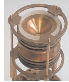
Fig. 2. Precision trap with hyperbolic electrodes. The characteristic trap dimensions are \rho_0 = 6.38 mm as the minimum radius and z_0 = 5.5 mm as the minimum distance from the trap center to the endcaps. Electrodes are isolated via customized sapphire pieces. The ring electrode is azimuthally segmented into an electrode pair for excitation ( 2 \times 40^\circ ) and detection ( 2 \times 140^\circ ).
